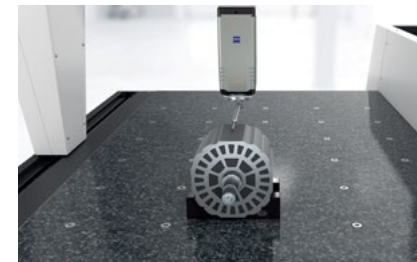
Rotor Dimensions Measuring on ZEISS CMM with Long Stylus System
