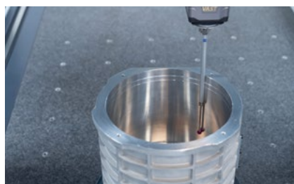
Measurement of Housing with ZEISS Tactile Scanning Technology
