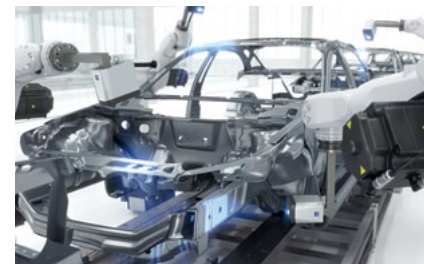
Optical inline inspection of the Battery Tray
