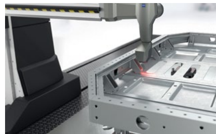
Optical Laser Triangulation Measurement of Battery Tray on ZEISS Horizon-tal Arm CMM
