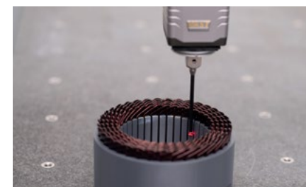
Measurement of Contour and Dimensional features together on one ZEISS CMM
