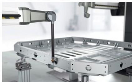
Tactile Measurement of Battery Tray on ZEISS Horizontal Arm CMM
