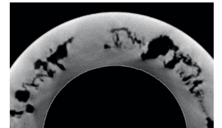
Cross section through the short circuit ring for porosity analysis
