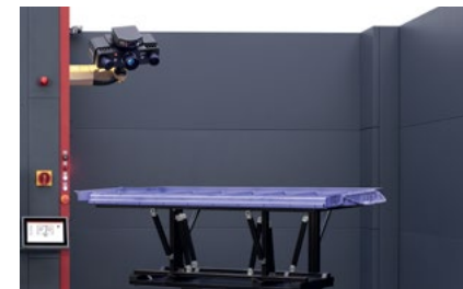
Optical measurements of a battery tray with a 3D measuring machine
